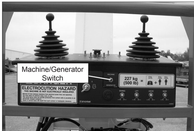
Figure 8.9 – Upper Control Panel Front
