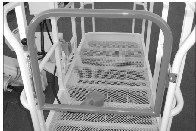
Figure 4.5 – Platform Swing Gate
